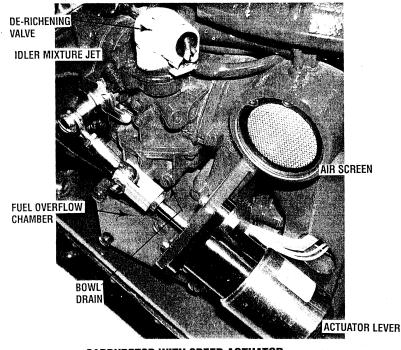
**CARBURETOR WITH SPEED ACTUATOR**
