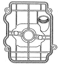
Apply the sealant to the shaded part. Shaded part (Part shown by slanted lines)
