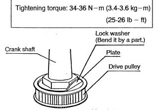
· After tightening the nut, bend up the lock washer
