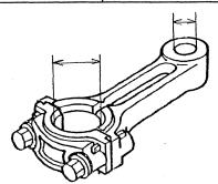
• Inner diameter of small end of connecting rod
