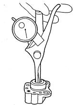
Inner diameter of valve guide
