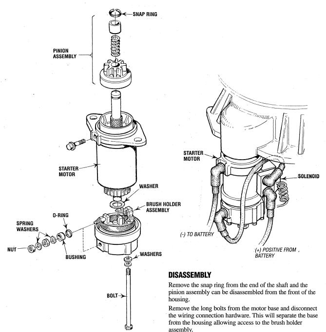
**NOTE:** This exploded view is to enable the customer to inspect clean and possiblty repair this starter motor, but parts are no longer available for this model motor.
