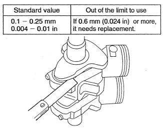
• Side clearance of crankshaft
