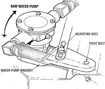
NOTE: The adjustment is the same for the FRESH WATER COOLED MODEL dual pumps.
