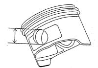
Clearance between piston pin and piston pin hole
