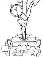
Oil clearance between cam shaft and holder
