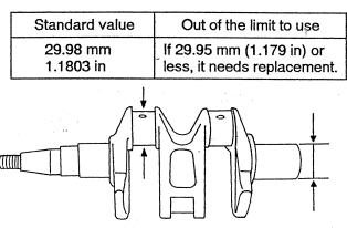
Outer diameter of crank shaft in metal bearing
