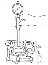
Diameter of piston pin hole
