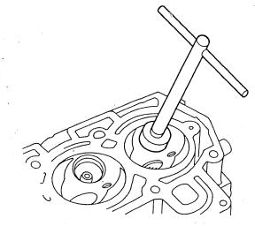
3) Apply Prussian Blue compound (or equivalent) evenly on the seat face. While turning the valve with the valve lapper, check face width between the valve and valve seat. If necessary, repair the face width with the valve seat cutter.
